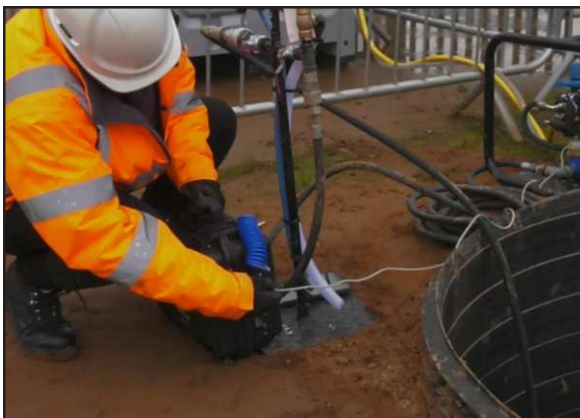
2. Connect the cable from the Flow Meter to the Pressure Logger.
