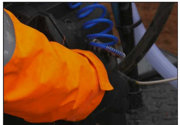
2. Connect the cable from the Flow Meter to the Pressure Logger.
