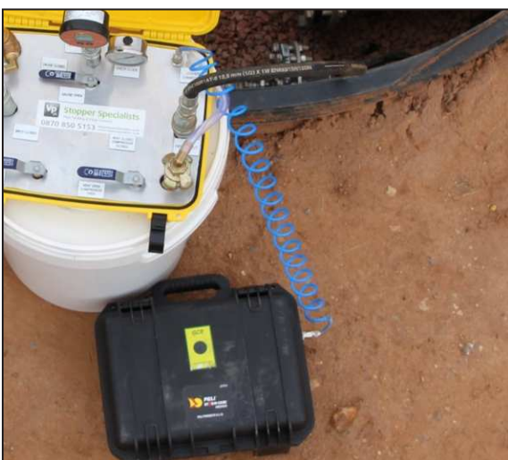
2. Connect the cable from the Flow Meter to the Pressure Logger.
